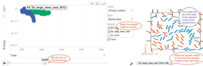
Fig. 3. Taken from the website, Glanz-Izrael (2013) - at left, energy of a 2d liquid crystal sample as a function of the temperature, and at right the visualization at a temperature value selected from the energy graph.
